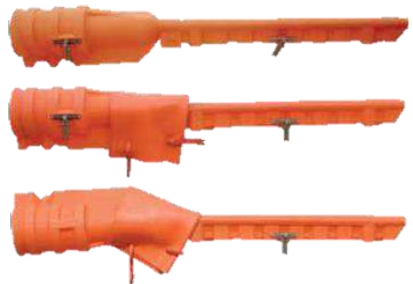
Deadend Cover couples with Conductor Cover using Hot Sticks or Rubber Gloves. (Must be used with Rubber Insulating Blanket)
