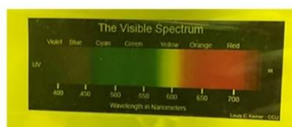
Visible spectrum through green arc flash faceshield
